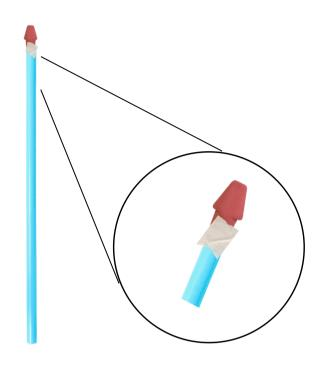
Slot the eraser onto the end of the straw and secure it with masking tape.
